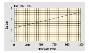
The curves are plotted using mineral oil with density of 0.86 kg/dm³ in compliance with ISO 3968.  $\Delta p$  varies proportionally with density.
