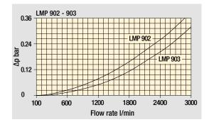
Bypass valve pressure drop
